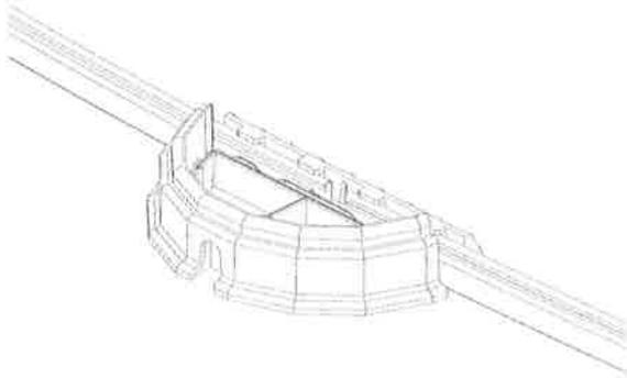
Assemble all bottom tracks to the bottom plates to form a perfect circle with a diameter and a radius in accordance to the chart
