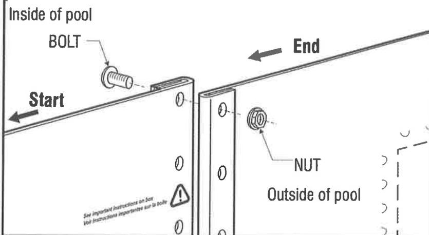
For proper grounding we suggest grounding the second wall bolt from the top of the wall seam. Use a 6 Gauge terminal and a 6 Gauge ground copper wire. Connect the wire to a 36" (1 m) grounding rod that will be inserted into the ground at least 36" (1 m) from the pool's perimeter. Please check the local electrical grounding codes for above ground pools in your county or state, as it varies from state to state.
