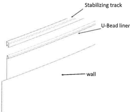
Hang the "U-Bead" liner on the top of the wall and install the round stabilisers to secure.
