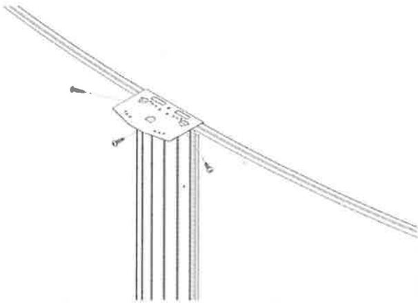
Install the joiner plates on top of each upright then install metal screws at the top of the support posts, making sure the support posts are perpendicular to the ground.
