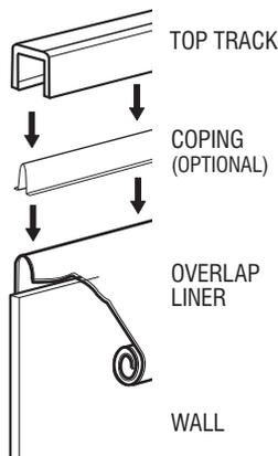
Installation detail of a bead liner with top track.
