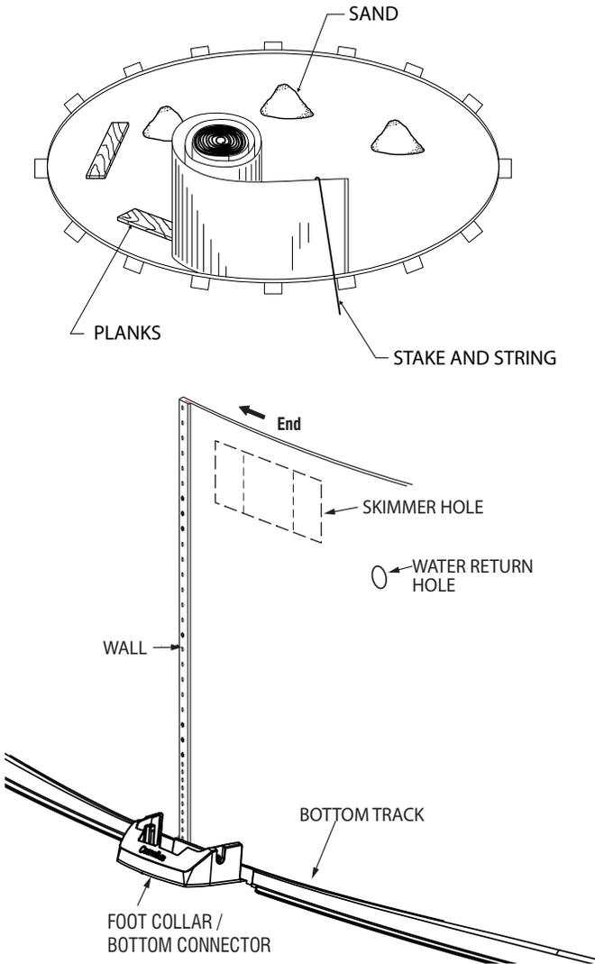
Begin inserting the wall into the bottom wall tracks in the middle of a joiner plate. At first, the wall is kept in place with one or two stakes and strings (or extra persons). One person uncoils the wall on a beam or a plank, while a second person inserts it in the bottom wall tracks. Do not uncoil more than 3 m (10') of wall before you install a support bar or stake and string to reinforce the structure.
