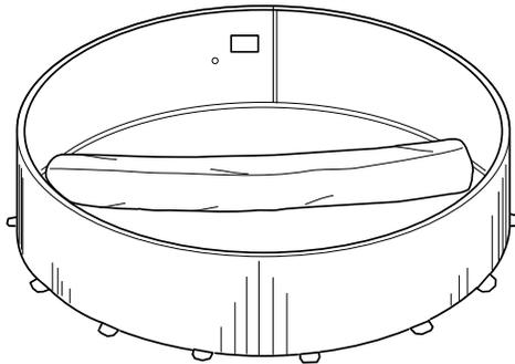
Lift up a section of the liner over the top of the wall leaving a 10 cm to 15 cm (4" to 6") fringe outside the wall. Secure the liner with a plastic coupler (sold separately). Install the top track on the wall then install the top plates on top of each upright.
