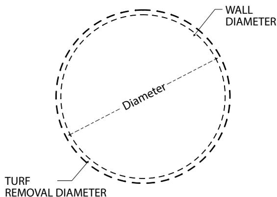
Drive a stake into the ground at the center of the site. Using a measuring tape, draw a circle 15 cm to 20 cm (6" to 8") longer in radius than the pool, depending on the width of the uprights (See Illustration 1.1).
