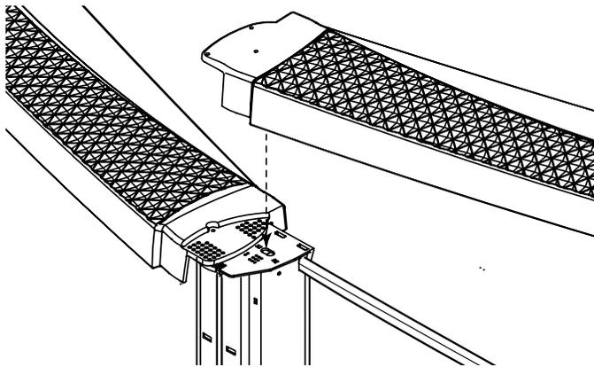
Place the top seats on the top of the uprights ensuring that the rod under the seat is inserted into the oblong holes in the top plate.
