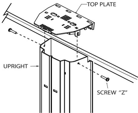
Install the top plate into the upright and secure with two (2) screws "Z" on each side.
