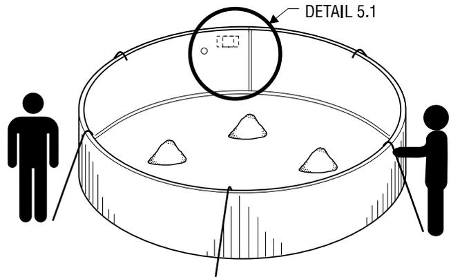
Once the wall is completely uncoiled, you may find that it is too long or that both ends do not meet by a few centimetres. If such is the case, adjust tracks and joiner plates until wall holes line up. If this does not work, roll up the wall again, check measurements as per chart 1.1, adjust tracks and plates, if applicable, and uncoil the wall again. If the spread is too wide, measure the wall and check it against the chart below.
